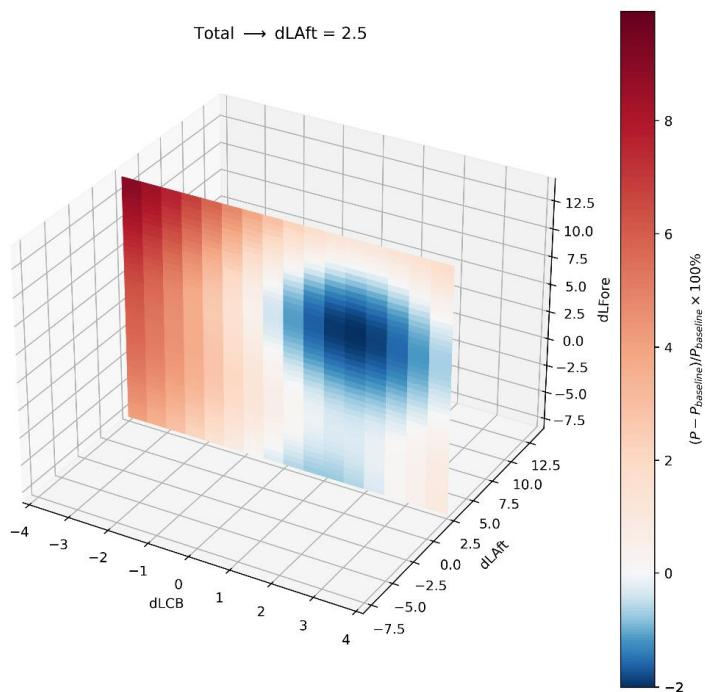
Images 1-2: The plot illustrates relative changes in weighted power, as predicted by the surrogate model. Colour gradients on the slice plane clarify variations within the design space for easier analysis.
