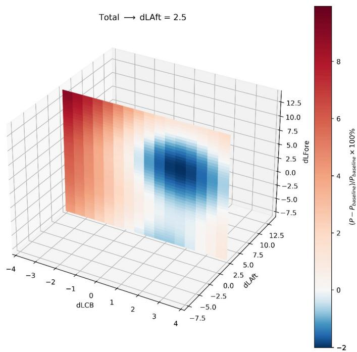
The plot illustrates relative changes in weighted power, as predicted by the surrogate model. Colour gradients on the slice plane clarify variations within the design space for easier analysis.
